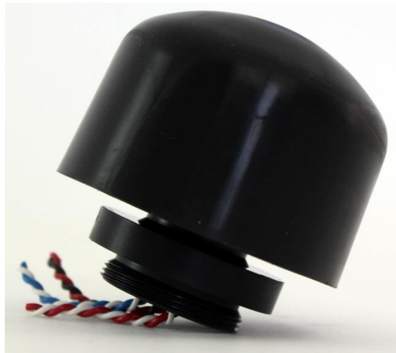
Figure 4: Photograph of a vector hydrophone built from five pressure hydrophones
