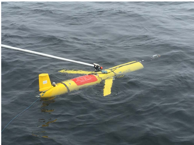
Fig. 1. Slocum glider equipped with externally mounted DMON
